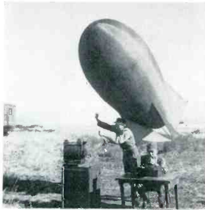
Airborne instruments check "ducting" effects at Ft. Huachuca, Arizona
